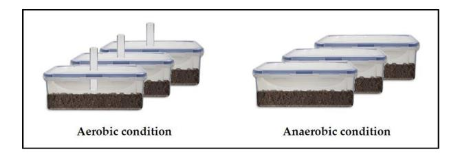
Figure S1. Illustration of the incubation boxes for aerobic and anaerobic conditions.
